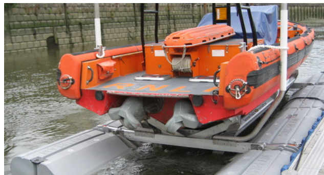
Chiswick reserve lifeboat now sits on a boat lift to protect its hull
